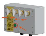
When the machine stop sequence is initiated, a signal from the machine control circuits starts the timer in the TDR unit. Once completed, the timer energizes the solenoid illuminating the green LED. By pushing the green button the keys can be released. These keys are taken by the operator to the machine
