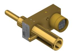
The KE lock is a one piece access interlock comprising of a main body and sliding bolt. The lock is designed to suit sliding doors of various sizes and thicknesses. The interlock is manufactured in brass and comes with the FS or Q lock type portions and is ideal for use in dry, non-corrosive environments where the lock is subject to medium to heavy use. Typical industries using the KE lock are automotive and steel production.
