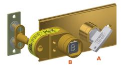
Key B is used as the personnel key and taken to the machine area. Key A stays trapped as long the catch is released and key B is free.
