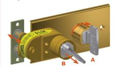
Inserting and turning key A in the bolt interlock enables the release of key B and the release of the catch. This will trap key A into the lock.
