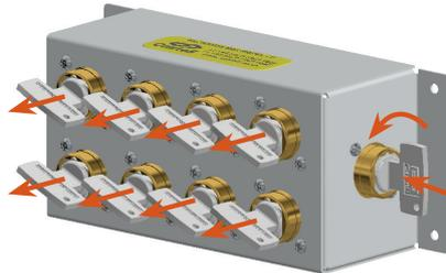
By inserting and turning the free end key in the Y key exchange box, you can release the trapped front keys in any order. Once the first key has been removed, the end key stays trapped. The released keys can be used in the access door locks to gain access to the hazardous area.
