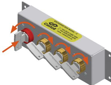
By inserting and turning the free key in the X key exchange box, trapped keys can be sequentially released. The released keys can be used in the access door locks to gain access to the hazardous area.
