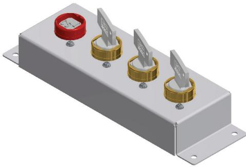
The X key exchange box is designed to enable the release of keys by the insertion of one or more primary key(s). The need for this type of product usually arises when there are multiple points of entry. The unit will generally be the link between the isolation locks and the access products. The product is supplied in an enclosure suitable for surface mounting and is available in a number of configurations and number of locks.
