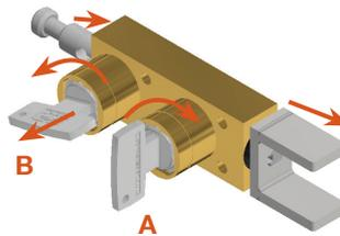
By inserting and turning key A in the KLC claw interlock, you can unlock the claw and manually extend the bolt. The claw now constrains the switch in the off position. Releasing key B will lock the claw in the extended position and trap key A. The released key B can be used as personnel key to gain access to the hazardous area via an access interlock.
