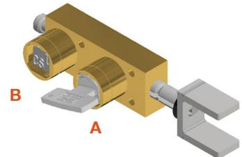
The switch cannot be switched on until key B is replaced in the KLC claw interlock, the bolt is retracted and key A released locking the claw in the retracted position.
