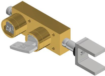
The KLC dual key claw interlock is a multi-key operated mechanical bolt interlock suitable for the control of electrical switchgear. The standard unit comes with a 16mm diameter bolt fitted with a claw that is used to control the rotation or movement of operating handles or toggles of electrical switchgear. The lock is manufactured in brass or stainless steel.
