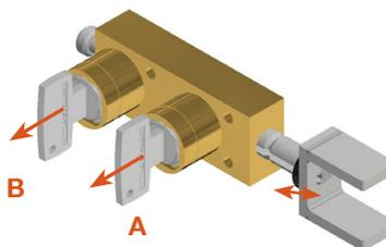
Driving the bolt, the claw is extended. Turning and releasing both keys will lock the claw in extended position constraining the switch in the off position. The released keys can be used as personnel keys to gain access to the hazardous area via an access interlock.
