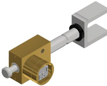
The KC Lock is a key operated mechanical bolt interlock suitable for the control of electrical switchgear. The standard unit comes with a 16 mm diameter bolt fitted with a claw, that is used to control the rotation or movement of the operating handles or toggles of electrical switchgear. The bolt length and claw dimensions are variable to suit the particular requirement. The lock is manufactured in brass or stainless steel.
