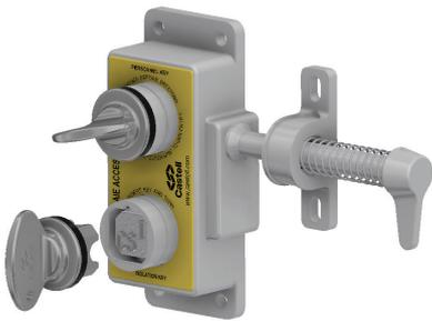
While the door is closed, the isolation key is free, the personnel key trapped in the AIE, and the bolt of the AIE is trapped in the mechanism.
