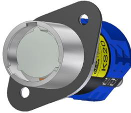
The KS20-MIS is a key driven electrical switch designed for machine control circuits. This type of isolator should be used for short term, off load isolation. The KS20-MIS is manufactured from chrome plated brass. The unit is able to be mounted into an existing panel or for surface mounting within its own IP65 rated enclosure.
